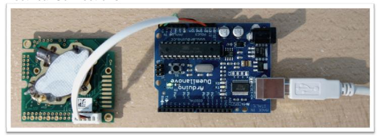
Interfacing with the sensor electrically is easy. Although the sensor runs at 3.3V it is tolerant of 5V logic levels. A direct electrical connection is possible using the Arduino's hardware I2C pins as follows:
